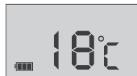
Diagram 7.6.4 - Battery Status This display indicates that the Transmitter unit is powered by batteries and indicates their power level.
