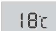
Diagram 7.6.3 - Normal Operation This display indicates the temperature and that the Transmitter unit is powered by the mains adaptor (no battery symbol).
