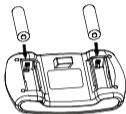
Fig 2: Place 2 batteries (AA/R6) into the compartment. Make sure the positive and negative ends of each battery match with the polarity indicators in the compartment.
